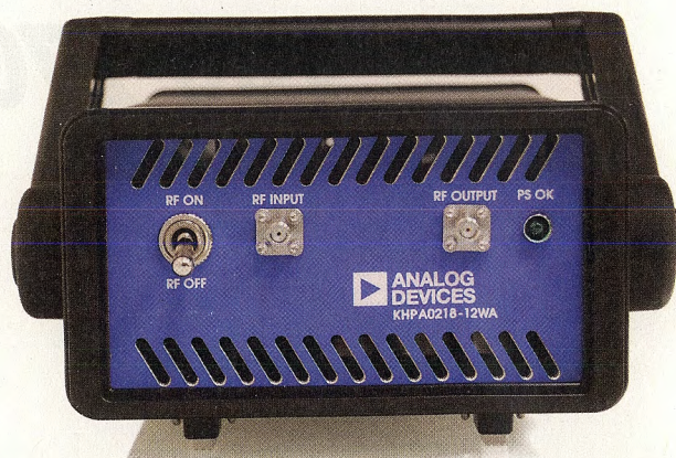
7. Across its full frequency range, this wideband 2- to 18-GHz power amplifier is capable of yielding 12-W CW output power.
