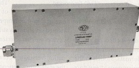
1. The LPAR50-dB-1WWP series of attenuators can handle 50-W average power and 2.5-kW peak power from 0.689 to 2.7 GHz while maintaining low passive-intermodulation (PIM) distortion. (Courtesy of MECA)
