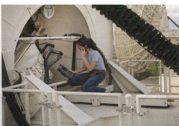
2. The light weight, small size, and multiple functions of the new FieldFox analyzers suit them for in-field testing, including at high-frequency satellite earth stations. (Courtesy of INTELSAT)
