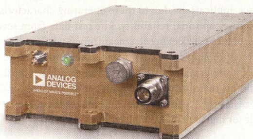
5. Up to 50-W CW output power from 2 to 18 GHz is possible with this amplifier.
